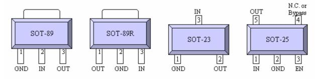
Figure 2 : pin configuration
