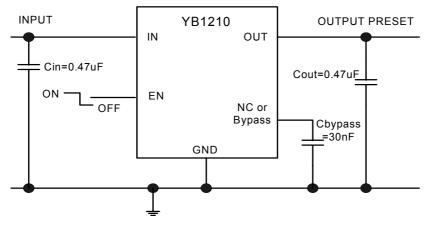
Figure 1-1. SOT-25 application circuit
