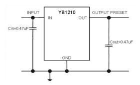
Figure 1-2. SOT-23 / SOT-89 application circuit
